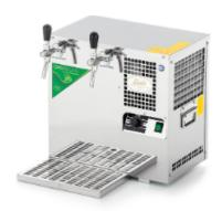
SODA is a professional device designed for producing chilled soda water by mixing H2O and CO2, also for dispensing of chilled beverage like water, lemonade, beer, wine nad cider. Its high output of up to 70 l/h make it suitable for professional use in restaurants, inns and bars.
