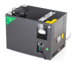
SODA AS 110 is a professional device designed for producing chilled soda water by mixing H2O and CO2, with the capability to cool two additional beverages (beer, fizzy drinks etc.). Its high output of 60-110 l/h make it suitable for professional use in restaurants, inns and bars
